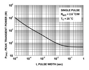
Figure 25. Single Pulse Maximum Power Dissipation
