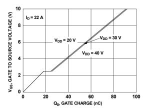
Figure 7. Gate Charge Characteristics
