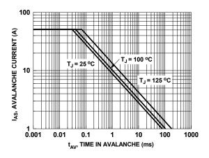
Figure 22. Unclamped Inductive Switching Capability
