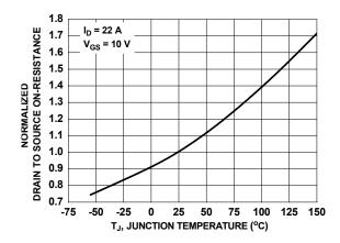
Figure 16. Normalized On-Resistance vs. Junction Temperature
