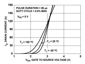
Figure 18. Transfer Characteristics
