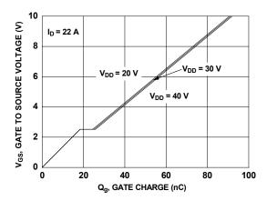
Figure 20. Gate Charge Characteristics
