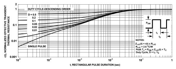
Figure 13. Junction-to-Case Transient Thermal Response Curve
