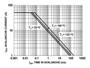
Figure 9. Unclamped Inductive Switching Capability
