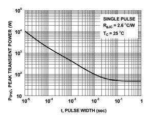
Figure 12. Single Pulse Maximum Power Dissipation
