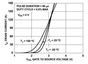
Figure 5. Transfer Characteristics
