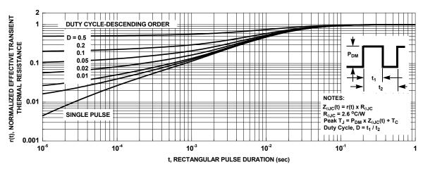
Figure 26. Junction-to-Case Transient Thermal Response Curve
