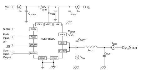
Figure 29. Block Diagram With V<sub>CIN</sub> Filter
