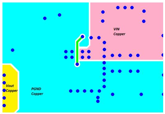
Figure 32. PCB Layout Example (Bottom View)
