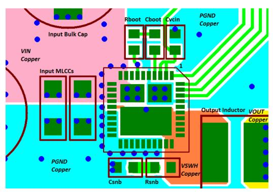
Figure 31. PCB Layout Example (Top View)
