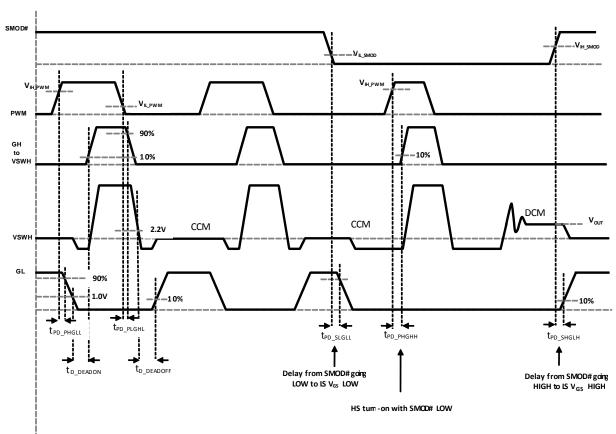
Figure 28. SMOD# Timing Diagram
