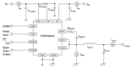
Figure 30. Power Loss Measurement
