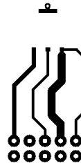
b) 118\text{ }^\circ\text{C/W} when mounted on a minimum pad of 2 oz copper
