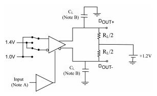
Note A: All LVTTL input pulses have frequency = 10MHz,  $t_R$  or  $t_F$  <= 2 ns Note B:  $C_L$  includes all probe and jig capacitances
