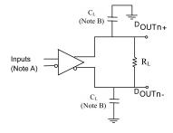
Note A: All LVDS input pulses have frequency = 10 MHz,  $t_{R}$  or  $t_{F}$   $\!<$  = 0.5 ns
