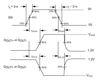
FIGURE 6. Enable and Disable AC Waveforms
