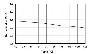
Figure 9. f<sub>MAX-CC</sub> vs. Temperature
