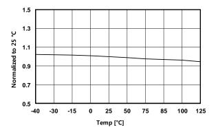
Figure 5. V<sub>DD-ON</sub> vs. Temperature
