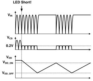
Figure 23. Waveforms in Short-LED Condition
