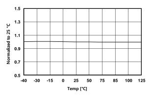
Figure 7. I<sub>DD-OP</sub> vs. Temperature
