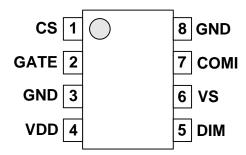
Figure 4. Pin Configuration
