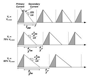
Figure 20. Primary and Secondary Current
