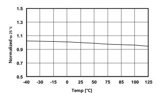
Figure 15. DS<sub>LOW</sub> vs. Temperature
