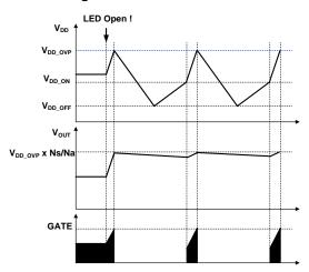
Figure 25. Waveforms in Open-LED Condition
