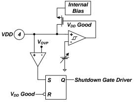
Figure 24. Internal OVP Block
