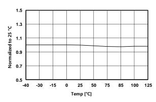
Figure 13. V<sub>OCP</sub> vs. Temperature
