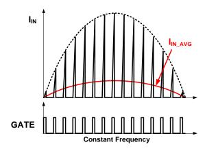
Figure 18. Input Current and Switching
