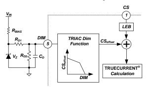
Figure 21. Dimming Control Schematic
