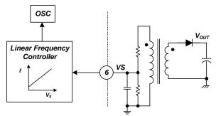
Figure 19. Linear Frequency Control
