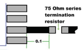
Figure 21 Distance from Device Pin to Series Termination Resistor
