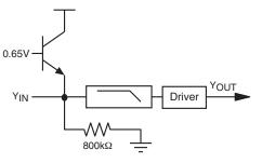
Figure 12. Input Clamp Circuit
