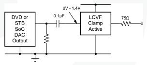
Figure 14. AC-Coupled Inputs, DC-Coupled Outputs
