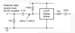
Figure 19. Biased SCART with AC-Coupled Outputs
