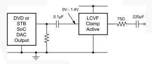
Figure 18. AC-Coupled Inputs, AC-Coupled Outputs
