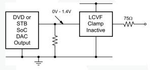
Figure 13. DC-Coupled Inputs and Outputs
