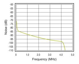
Figure 21. Noise vs. Frequency CV<sub>OUT</sub>
