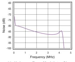
Figure 11. Noise vs. Freq. Modulator Channel
