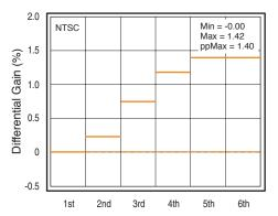
Figure 17. Differential Gain, CVOUT
