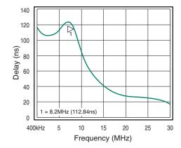
Figure 6. Group Delay vs. Frequency CV<sub>OUT</sub>
