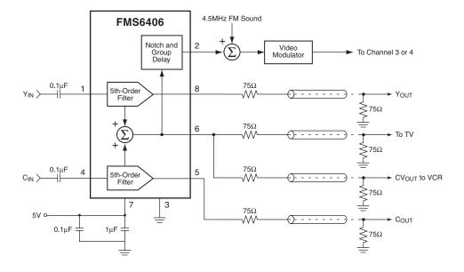
Figure 23. DC-Coupled Application Diagram
