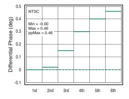
Figure 18. Differential Phase, CV<sub>OUT</sub>
