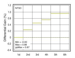
Figure 15. Differential Gain, COUT
