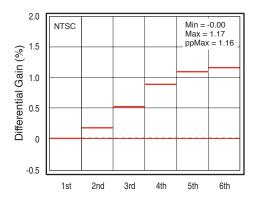
Figure 13. Differential Gain, VOUT
