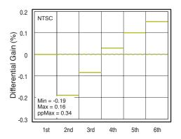
Figure 9. Differential Gain, MODOUT
