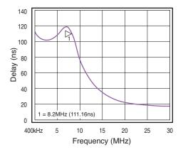
Figure 4. Group Delay vs. Frequency Cout
