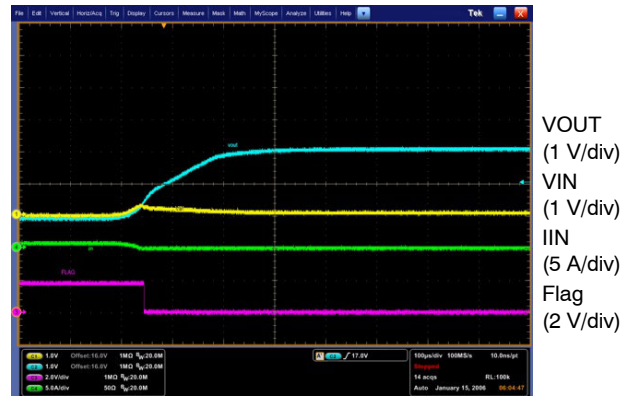
Figure 15. TRCB Behavior for Rout = 20 Ω (FLTb was configured active)
