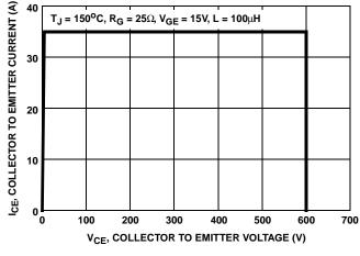
FIGURE 2. MINIMUM SWITCHING SAFE OPERATING AREA
