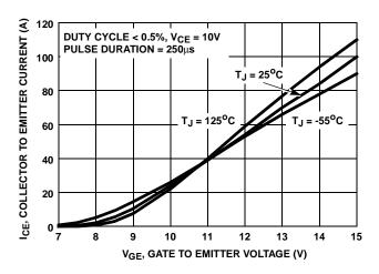
FIGURE 13. TRANSFER CHARACTERISTIC
