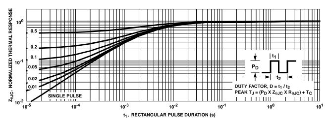
FIGURE 19. IGBT NORMALIZED TRANSIENT THERMAL RESPONSE, JUNCTION TO CASE
