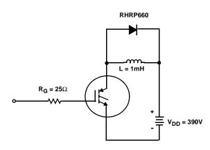
FIGURE 20. INDUCTIVE SWITCHING TEST CIRCUIT
