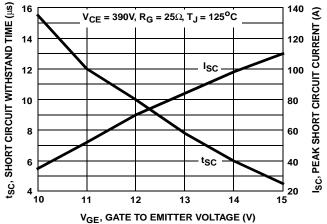
FIGURE 4. SHORT CIRCUIT WITHSTAND TIME
