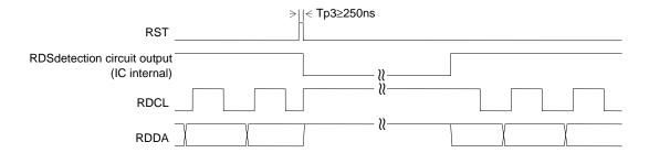
Note: RDCL and RDDA outputs keep high level after input of RST until RDS detection circuit output is detected.
