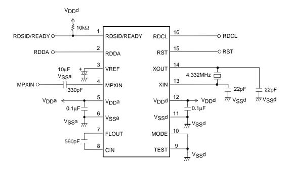
Note: If the RST pin is unused, it must be connected to ground.
