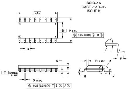
NOTES: 1. DIMENSIONING AND TOLERANCING PER ANSI Y14.5M, 1982. 2. CONTROLLING DIMENSION: MILLIMETER. 3. DIMENSIONS A AND B DO NOT INCLUDE MOLD PROTRUSION. 4. MAXIMUM MOLD PROTRUSION 0.15 (0.006) PER SIDE. 5. DIMENSION D DOES NOT INCLUDE DAMBAR PROTRUSION. ALLOWABLE DAMBAR PROTRUSION SHALL BE 0.127 (0.005) TOTAL IN EXCESS OF THE D DIMENSION AT MAXIMUM MATERIAL CONDITION.
