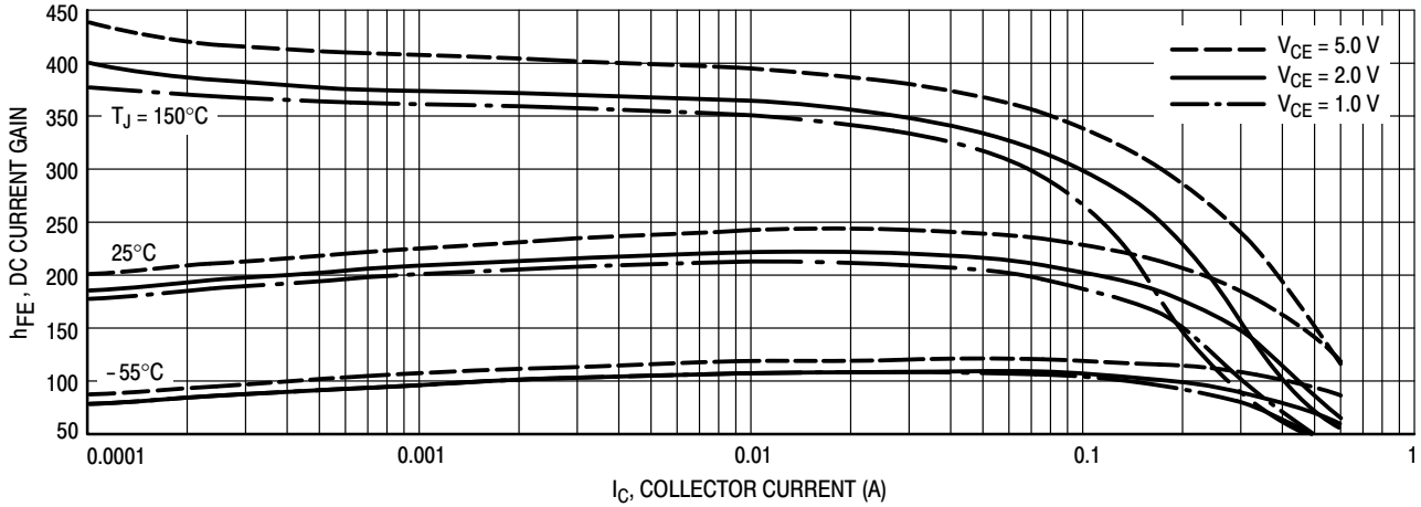
Figure 12. DC Current Gain
