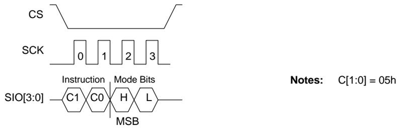
**Figure 11. QUAD Read Mode Register Sequence (RDMR)**
