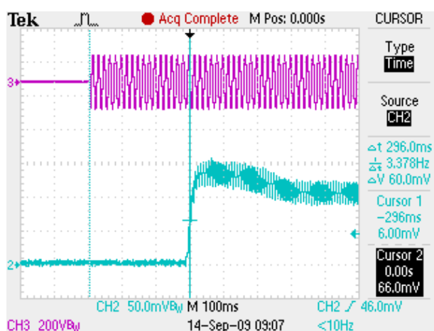
Figure 37. Start up Characteristic with 36.9 V, 350 mA Load
