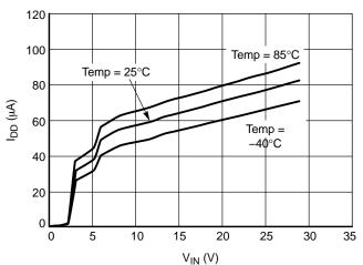
Figure 8. Quiescent Current vs. Vin, Over Temperature
