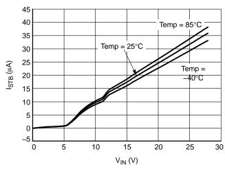
Figure 6. Standby Current vs. Vin, Over Temperature
