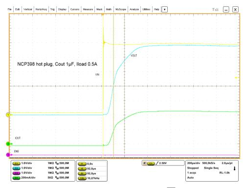
Figure 11. Hot Plug On Load, Vin: yellow, Vout: blue, EN: pink, IOUT: green
