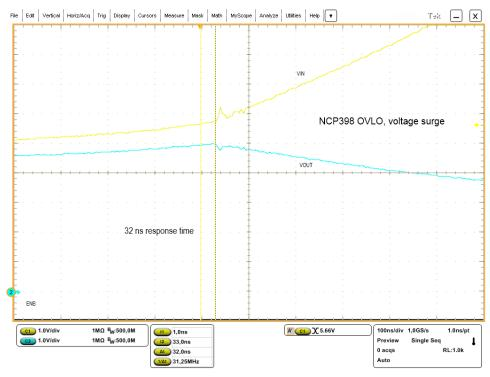
Figure 15. NCP398 Overvoltage Time Response, Vin: yellow, Vout: blue
