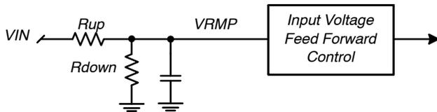
Figure 5. Ramp Feed Forward Circuit
