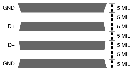
Figure 22. Typical Arrangement of Signal Tracks
