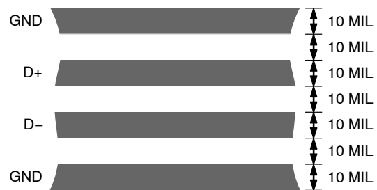
Figure 17. Arrangement of Signal Tracks
