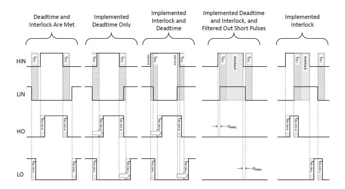
Figure 6. Deadtime, Interlock and Output Minimum Pulse Width
