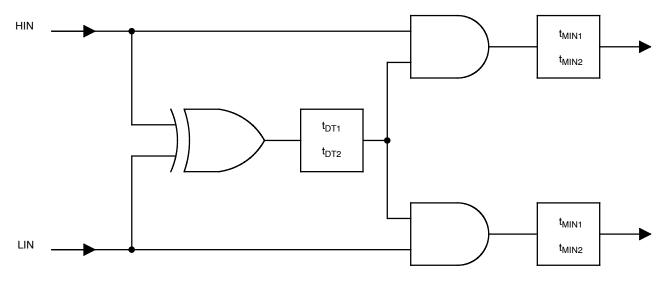
Figure 7. Input Circuit
