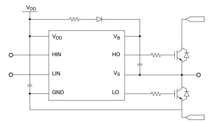
Figure 2. Simplified Application Schematics
