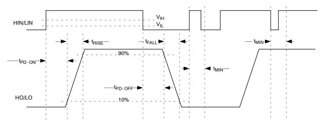
Figure 3. Propagation Delay, Rise and Fall Time
