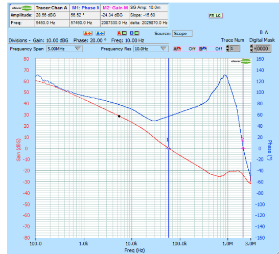
Figure 73. Bode Plot NCV6323FxmLMTW12TBG L = 1.0 μH – COUT = 100 μF
