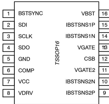
Figure 10. Pin Connections – TSSOP16 (Top View)
