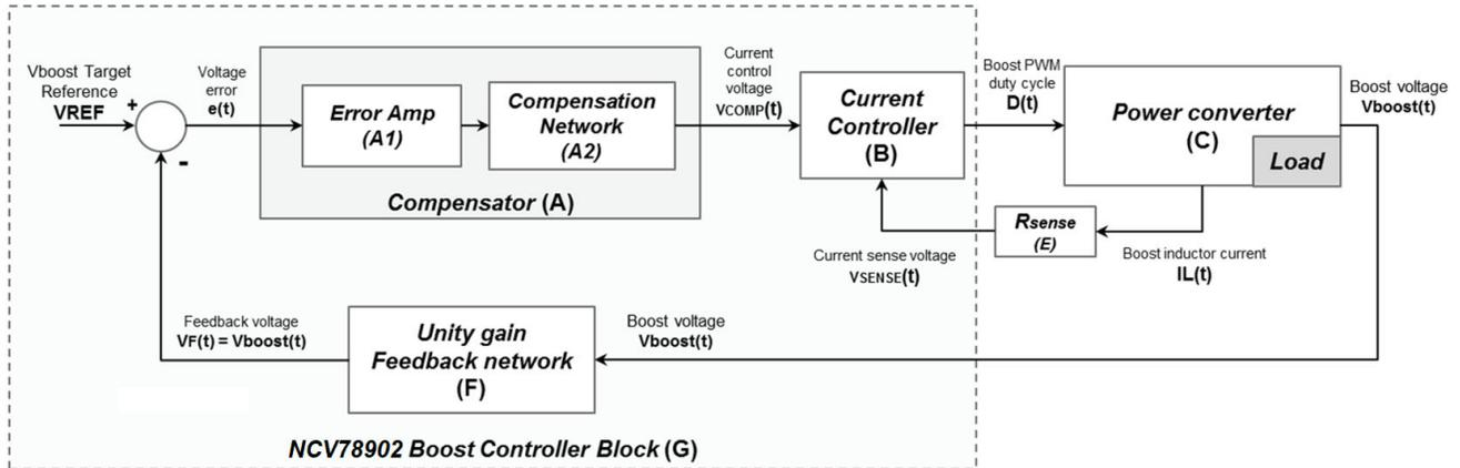
**Figure 13. NCV78902 Boost Control Loop – Principle Block Diagram**
