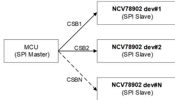
Figure 23. SPI Star Connection
