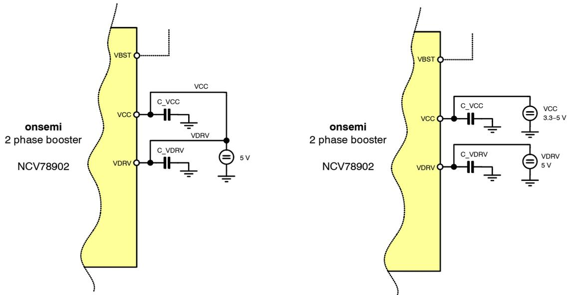
**Figure 7. Application Schematic – SUPPLY Connection Possibilities**
