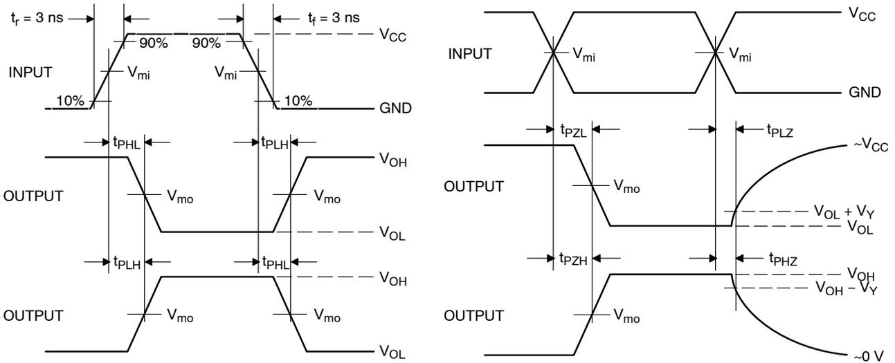
**Figure 4. Switching Waveforms**
