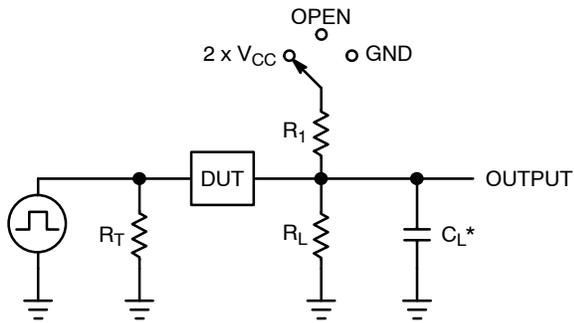
$C_L$  includes probe and jig capacitance
