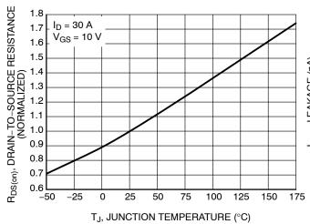
Figure 5. On-Resistance Variation with **Temperature**
