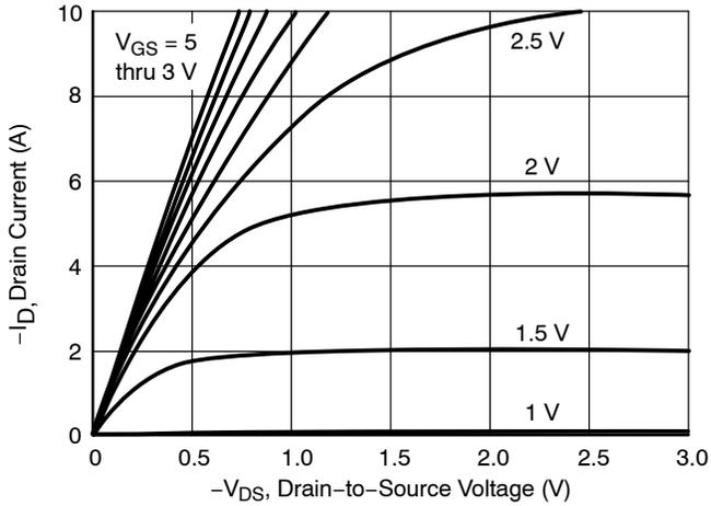
Figure 1. Output Characteristics
