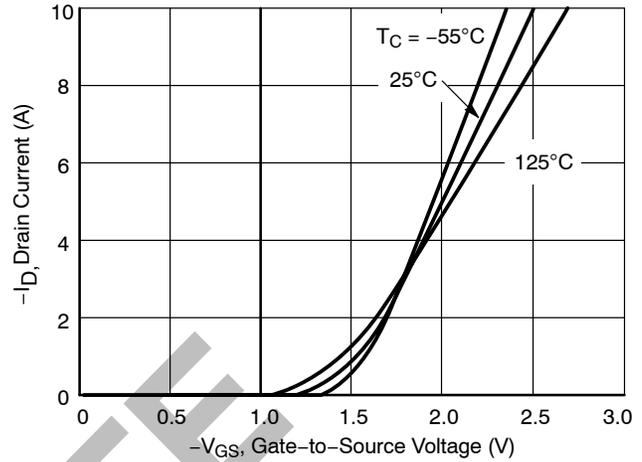
Figure 2. Transfer Characteristics
