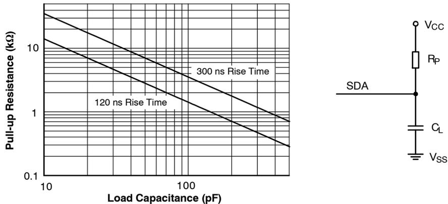
**Figure 2. Maximum Pull-up Resistance vs. Load Capacitance**
