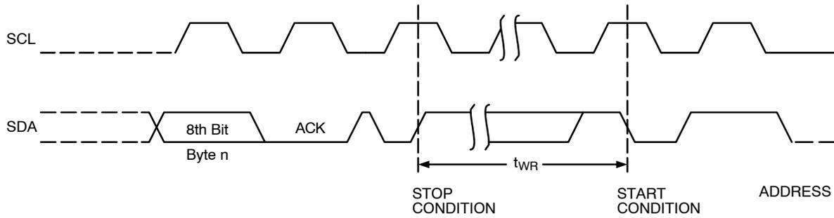
Figure 8. Write Cycle Timing
