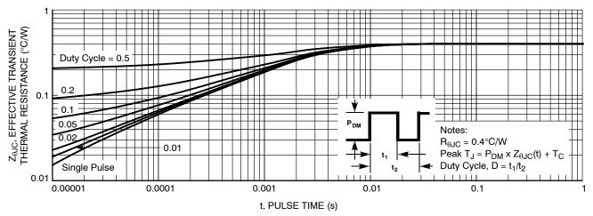
Figure 8. Junction-to-Case Transient Thermal Response Curve
