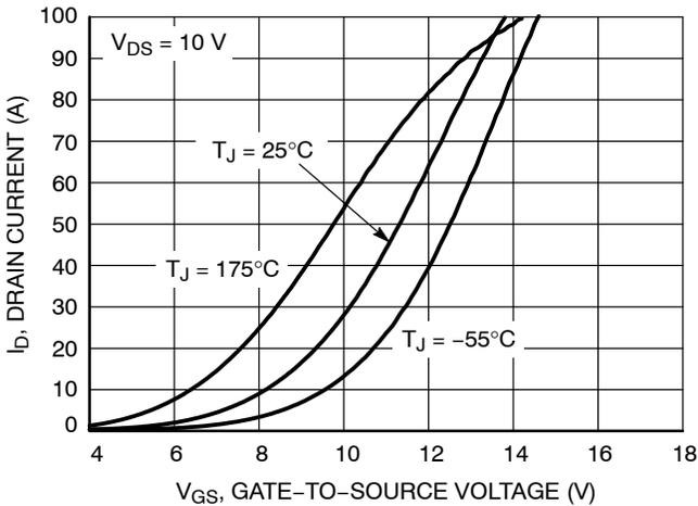
Figure 5. Transfer Characteristics
