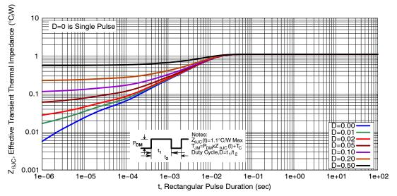
Figure 15. Transient Thermal Response
