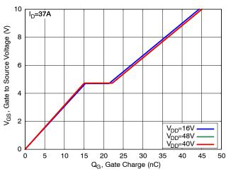
Figure 8. Gate Charge Characteristics
