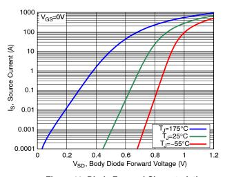
Figure 10. Diode Forward Characteristics
