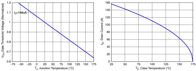
Figure 13. Gate Threshold Voltage vs. Junction Temperature
