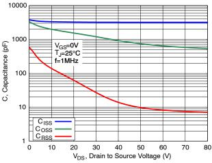
Figure 7. Capacitance Characteristics
