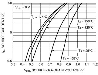
Figure 10. Diode Forward Voltage vs. Current
