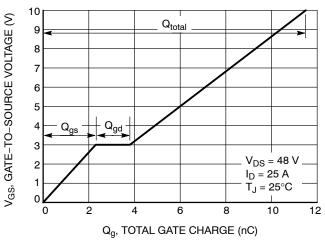
Figure 8. Gate-to-Source vs. Total Charge
