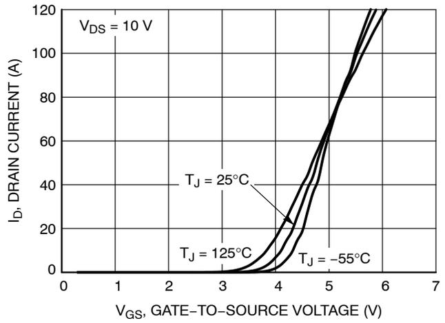
Figure 2. Transfer Characteristics
