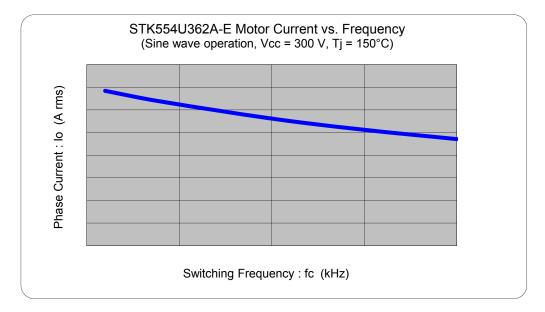
Fig.11 Maximum sinusoidal phase current as function of switching frequency at Tc = 100°C, V<sub>CC</sub> = 300 V
