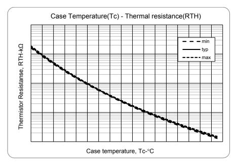
Fig.9 Variation of thermistor resistance with temperature
