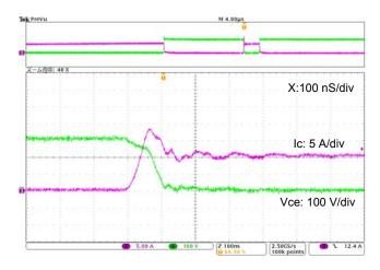
Fig. 12 IGBT Turn-on. Typical turn-on waveform at Tc = 100°C, V<sub>CC</sub> = 300 V, Ic = 10 A
