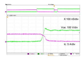
Fig. 13 IGBT Turn-off. Typical turn-off waveform Tc = 100°C, V<sub>CC</sub> = 300 V, Ic = 10 A
