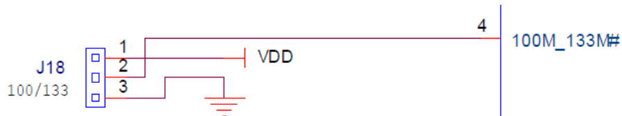
Figure 6. 100M_133M# Pin Schematic Configuration
