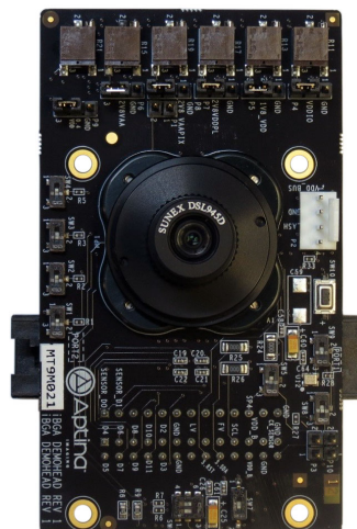
Figure 1. MT9M021 Evaluation Board
