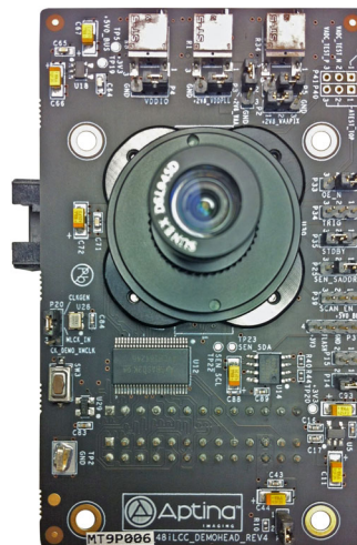
Figure 1. MT9P006 Evaluation Board
