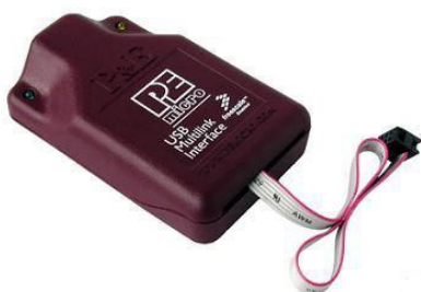
Figure 22. PEmicro USB Multilink BDM module (Discontinued)
