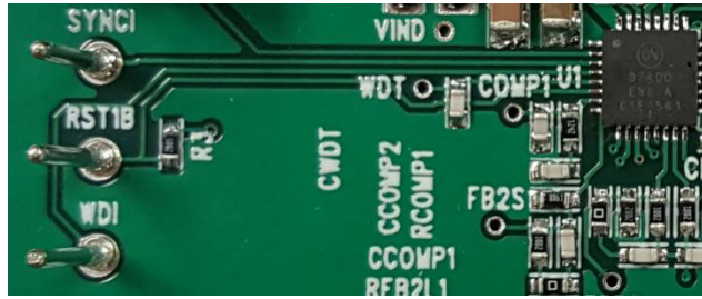
Figure 14. NCV97400 Watchdog Pins
