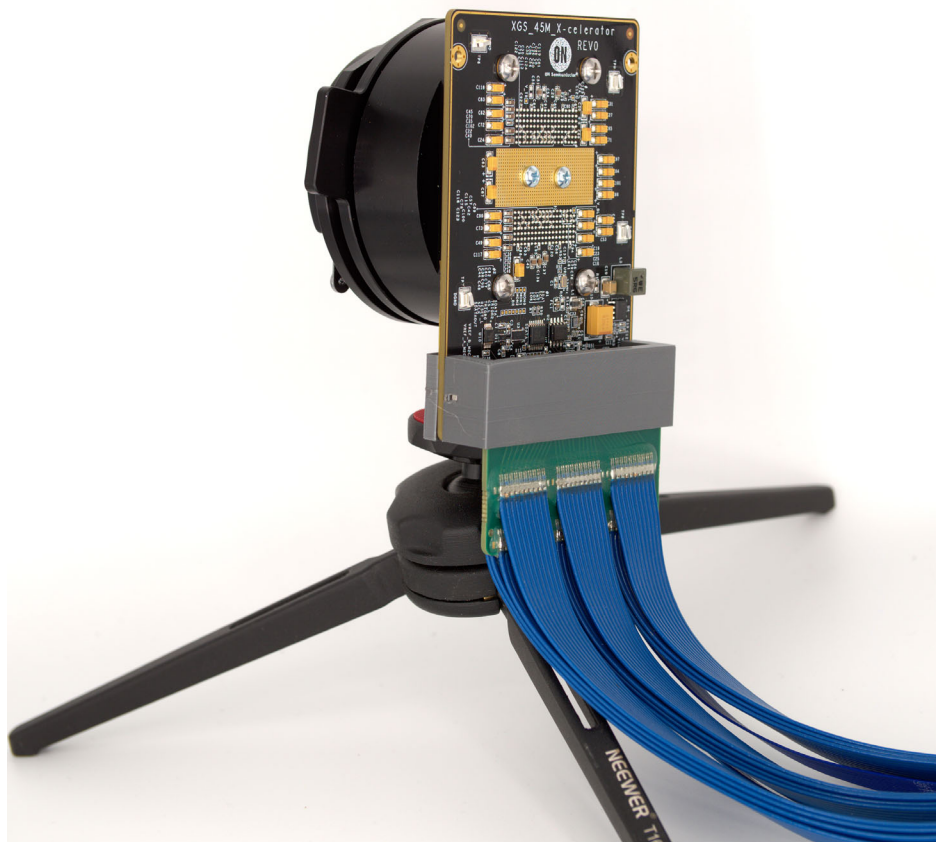
Figure 10. XGS 45000 Development Kit Setup
