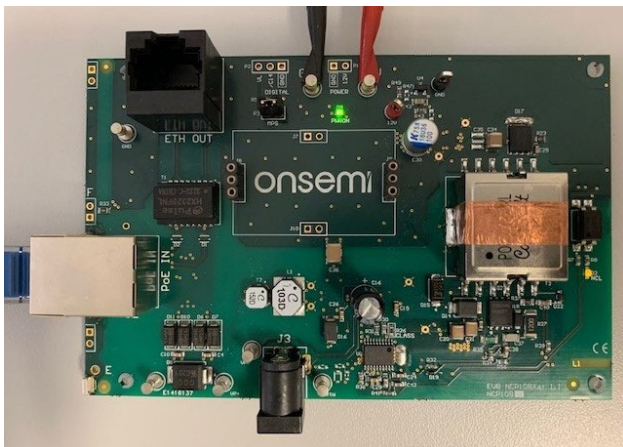
Figure 1. Operational NCP1081REF12VC4GEVB showing Basic Interconnections
