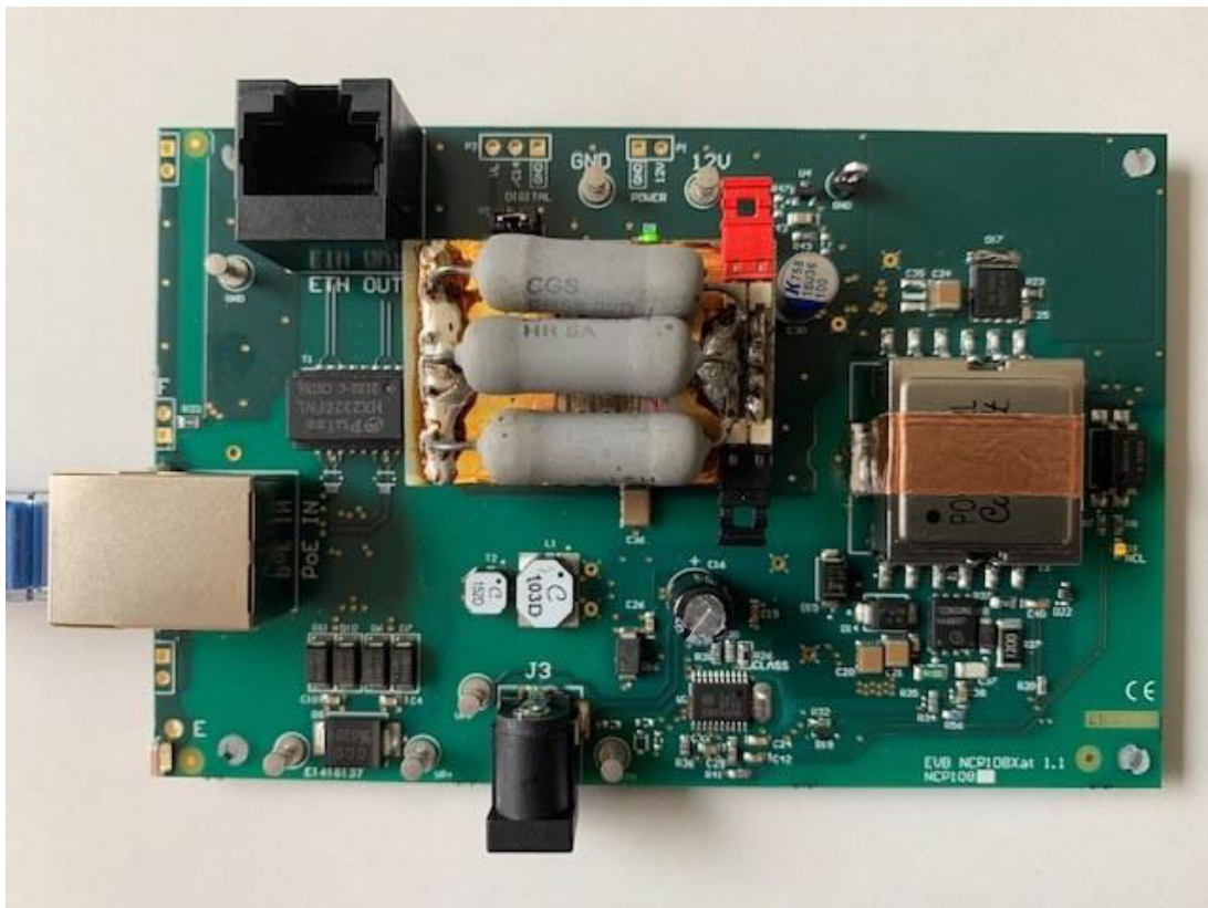
Figure 13. Emission Test DUT: NCP1081REF12VGEVB with 7.3 \Omega Load
