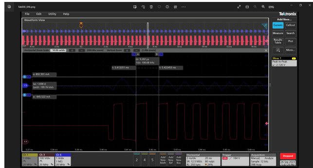
Figure 20. Skip Mode @ 50 V/0.06 A Load
