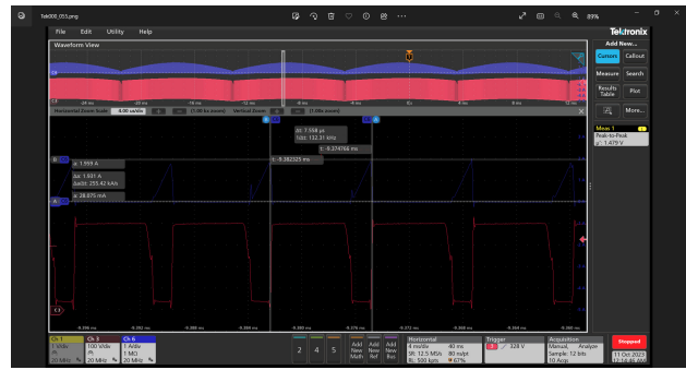
Figure 18. 230 Vac Input & Full Load
