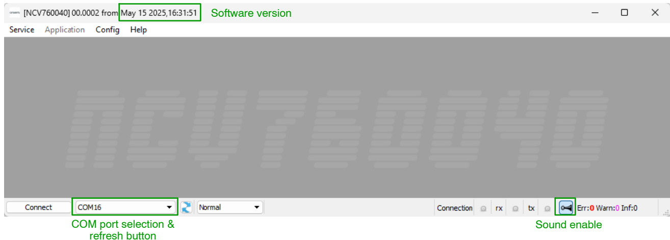
Figure 4. NCV760040 Controller Framework
