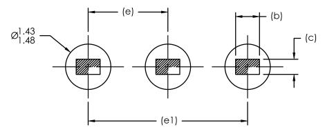
NOTE: LAND PATTERN AND THROUGH HOLE DIMENSIONS SERVE ONLY AS AN INITIAL GUIDE. END-USER PCB DESIGN RULES AND TOLERANCES SHOULD ALWAYS PREVAIL.
