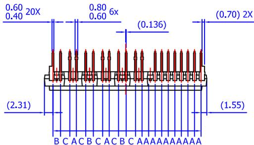
LEAD PITCH (TOLERANCE : ±0.30)
