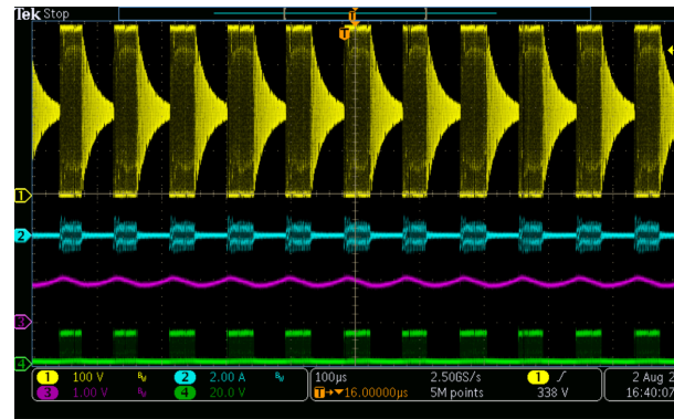
Figure 32. Waveform at 115 Vac and 48 V 0.5 A (ch1-Vllc-sw, ch2-lp, ch3-Vfb, ch4-Vldrv)
