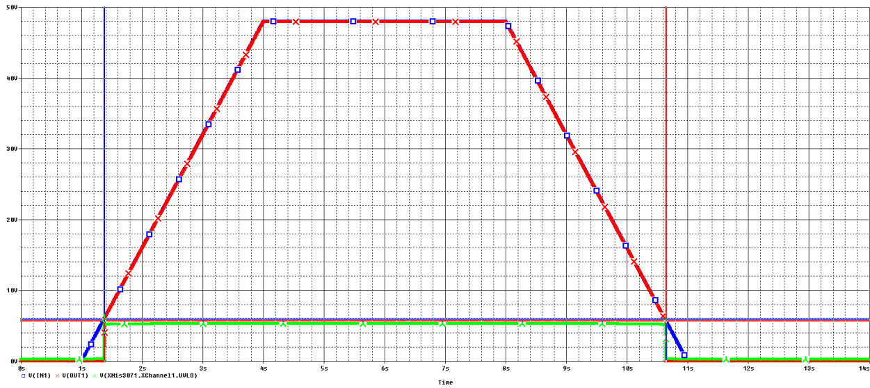
Figure 5. Slow Input Ramp to Show UVLO
