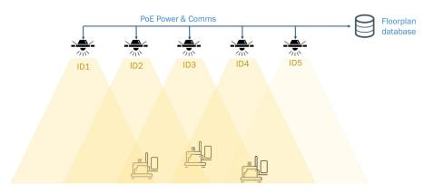
Figure 4. LED Ballast with Unique ID
