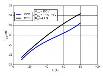
Figure 28. Typical On Switching Times vs. IC
