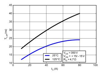
Figure 31. Typical Off Fall Times vs. IC
