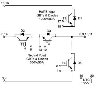
Figure 1. Schematic Diagram
