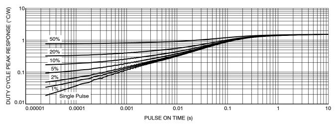
Figure 19. Diode Transient Thermal Impedance
