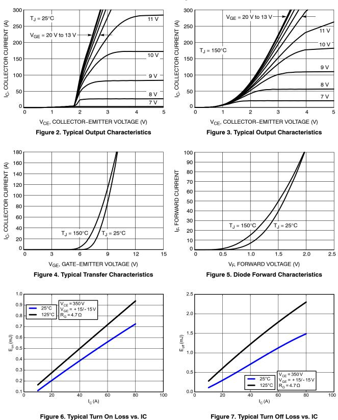
**TYPICAL CHARACTERISTICS – Half Bridge IGBT and Neutral Point Diode**
