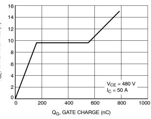
Figure 37. Gate Voltage vs. Gate Charge
