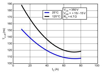
Figure 29. Typical Off Switching Times vs. IC
