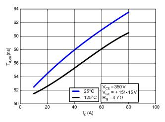
Figure 8. Typical On Switching Times vs. IC
