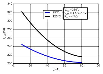
Figure 9. Typical Off Switching Times vs. IC
