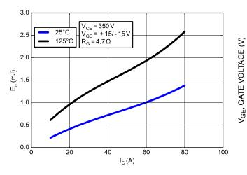
Figure 36. Typical Reverse Recovery Energy vs. IC
