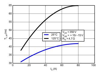
Figure 11. Typical Off Fall Times vs. IC
