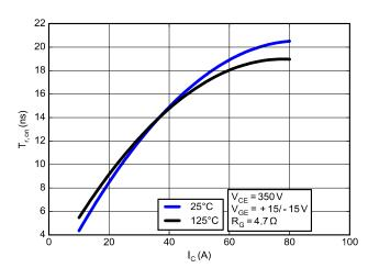
Figure 30. Typical On Rise Times vs. IC
