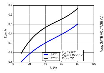
Figure 16. Typical Reverse Recovery Energy vs. IC
