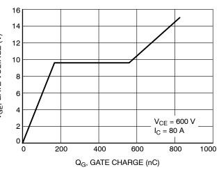
Figure 17. Gate Voltage vs. Gate Charge
