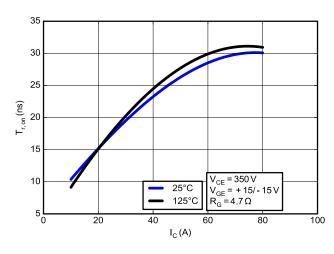
Figure 10. Typical On Rise Times vs. IC
