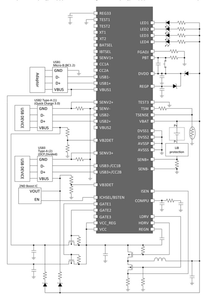
Type-C (Sink: BC1.2, Source: Quick Charge 3.0 HVDCP) + Type-A (Source: DCP and Divided mode)
