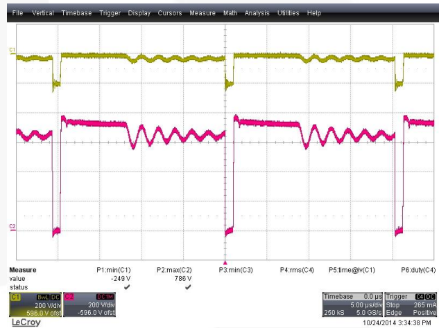
Figure 45. V DS =786 V, V DIODE =249 V, Steady-State, Full-Load Condition, 460 V AC , (CH1: V DIODE (200 V/div), CH2: V DS (200 V/div), Time: 5 μs/div)
