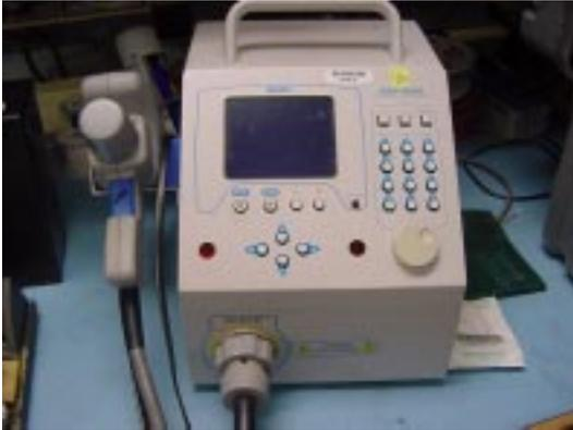
Figure 9. ESD Generator, NoiseKen ESS-2000
