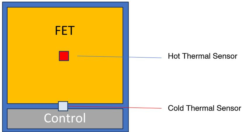
**Figure 9. Sensing Elements in Differential Thermal Shutdown**
